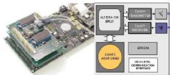
Fig. 9. Block diagram and application manager prototype.
