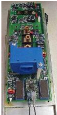
Fig. 7. Prototype of phase leg module integrated with hardware manager.
