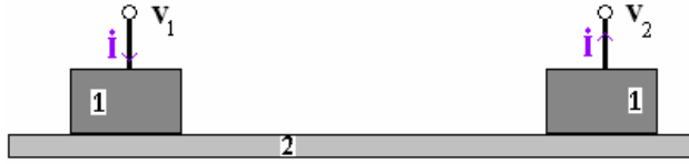
Fig. 3. The two contacts measurement method
