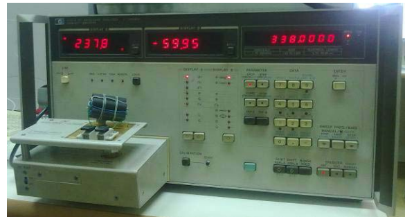
Fig. 6. Measurement setup for measuring bundle impedances using HP 4191A impedance analyzer
