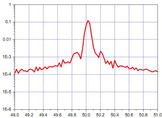
Fig. 4. The faulty cage with several cracked and broken rotor bars, cage current spectrum (relative amplitude versus frequency) around fundamental frequency (50 Hz)
